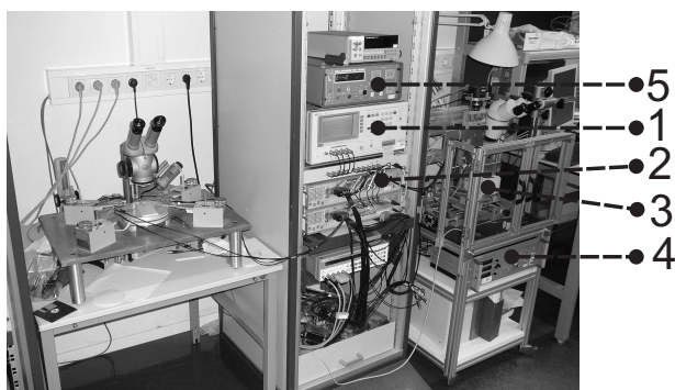
Figure 4.14 – Automated impedance measurement setup with 1) a HP4284a precision LCR meter, 2) a Keithley 708 switching system, 3) PI Physik Instrumente C-560 stepping motor controller, 4) wafer chuck and probe card, and 5) Sefelec PM04 milliohm meter.
